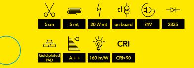
DDS605 is a 20W meter led strip with 140 led 2835 per meter. To produce our indoor flexible LED strips, we use 3-step McAdam LEDs, gold plated flexible double side PCB and constant current control inside the LED strip. Thermal conductive adhesive tape guarantees perfect heat transfer to the mounting suface. All of our product features guarantee
