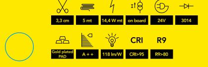
DDS535 is a 14W meter led strip with 210 led 3014 per meter. To produce our indoor flexible LED strips, we use 3-step McAdam LEDs whit high CRI and high R9, gold plated flexible double side PCB and constant current control inside the LED strip. Thermal conductive adhesive tape guarantees perfect heat transfer to the mounting suface.
